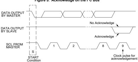
Figure 5. Acknowledge on the I<sup>2</sup>C Bus
