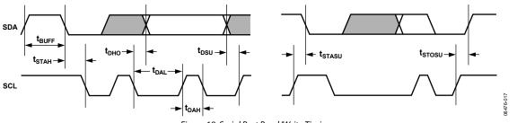
Figure 18. Serial Port Read/Write Timing
