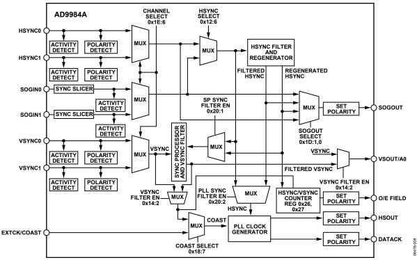
Figure 9. Sync Processing Block Diagram
