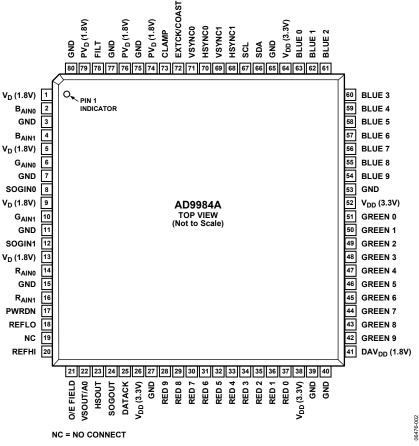
Figure 2. 80-Lead LQFP Pin Configuration
