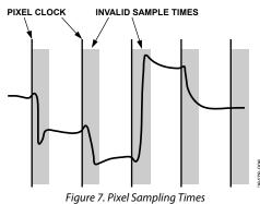
Any jitter in the clock reduces the precision of the sampling time and it must also be subtracted from the stable pixel time. Considerable care has been taken in the design of the AD9984A clock generation circuit to minimize jitter. The clock jitter of the AD9984A is low in all operating modes, making the reduction in the valid sampling time due to jitter negligible.
