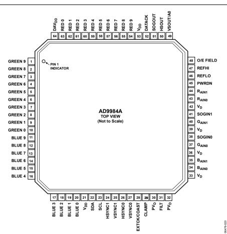
Figure 3. 64-Lead LFCSP Pin Configuration
