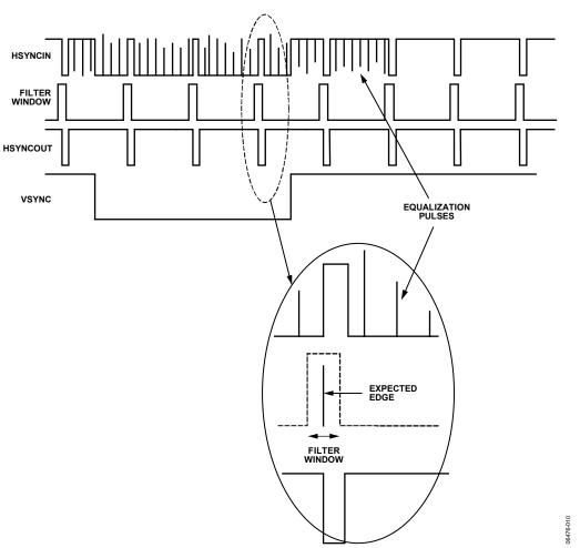
Figure 11. Sync Processing Filter
