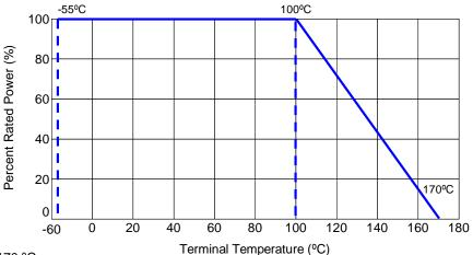
Operating temperature range of -55 to 170  $^{\circ}$ C. Storage condition: 5 ~ 35  $^{\circ}$ C, humidity of 40 ~ 75%.
