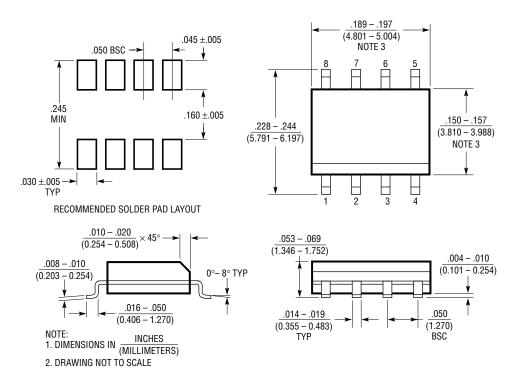
THESE DIMENSIONS DO NOT INCLUDE MOLD FLASH OR PROTRUSIONS. MOLD FLASH OR PROTRUSIONS SHALL NOT EXCEED .006" (0.15mm)
