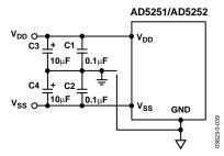
Figure 39. Power Supply-Bypassing Configuration
