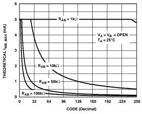
Figure 22. AD5252 IwB\_MAX vs. Code
