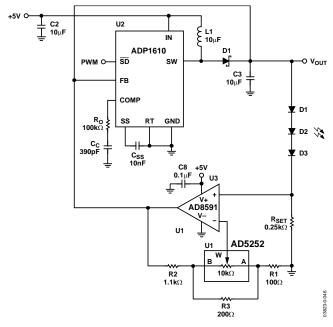
Figure 46. High Power, Adjustable LED Driver
