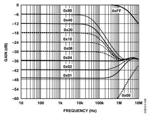
Figure 16. AD5252 Gain vs. Frequency vs. Code,  $R_{AB}=100~k\Omega$  ,  $T_A=25^{\circ}C$
