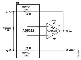
Figure 45. Current-Sensing Amplifier
