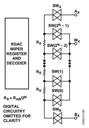
Figure 40. Equivalent RDAC Structure
