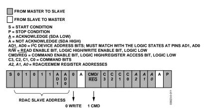
Figure 31. RDAC Quick Command Write (Dummy Write)
