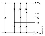
Figure 38. Maximum Terminal Voltages Set by V<sub>DD</sub> and V<sub>SS</sub>
