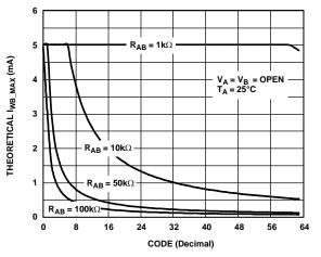
Figure 21. AD5251 IwB\_MAX vs. Code
