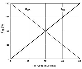
Figure 42. AD5251 R<sub>WA</sub>(D) and R<sub>WB</sub>(D) vs. Decimal Code
