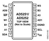
Figure 2. Pin Configuration
