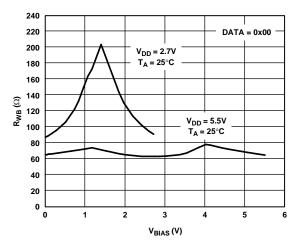
Figure 9. Wiper Resistance vs. V<sub>BIAS</sub>
