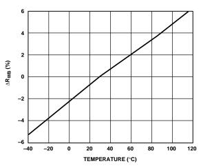
Figure 10. Change of R<sub>WB</sub> vs. Temperature
