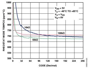
Figure 11. AD5252 Rheostat Mode Tempco ΔR<sub>WB</sub>/ΔT vs. Code
