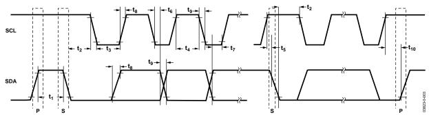
Figure 23. I<sup>2</sup>C Interface Timing Diagram
