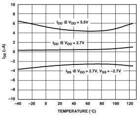
Figure 7. Supply Current vs. Temperature
