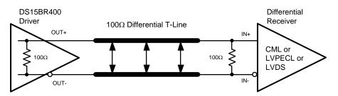
Figure 14. Typical DS15BR400 Output DC-Coupled Interface to an LVDS, CML or LVPECL Receiver
