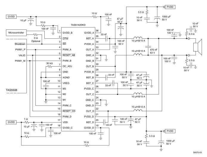
Figure 17. Typical Differential (2N) PBTL Application With AD Modulation Filters
