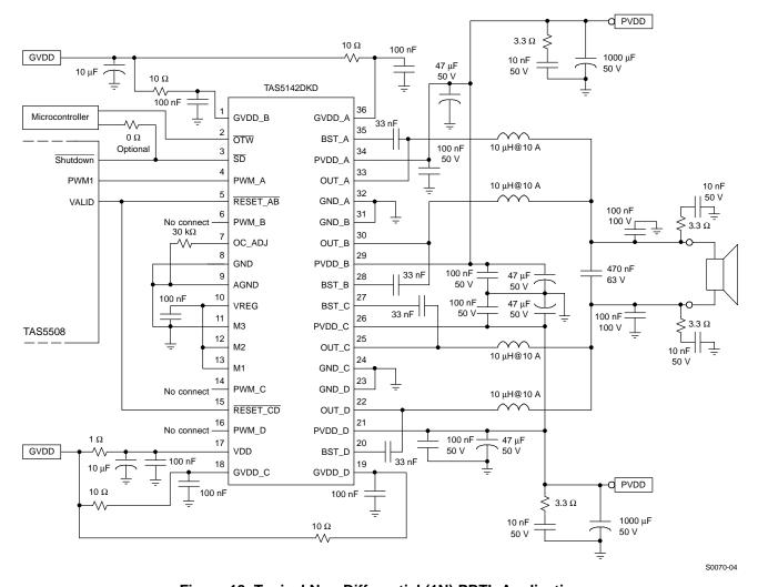
Figure 18. Typical Non-Differential (1N) PBTL Application
