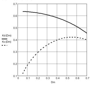
Fig. 1. Conduction Loss Coefficients K<sub>c</sub> and K<sub>d</sub>
