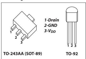
**Drain** – This is a drain terminal of the output switching MOSFET and a linear regulator input.
