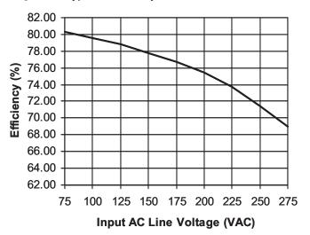
Figure 5. Typical Efficiency
