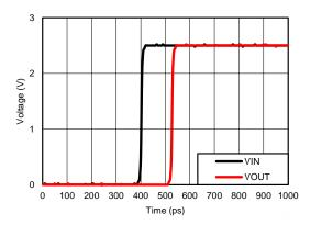
Figure 6. Propagation Delay ( $t_{pd}$ ) Simulation Result at  $V_{CC} = 2.5 \text{ V}$ .
