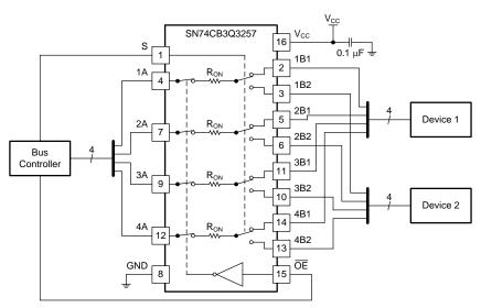
Figure 5. Typical Application of the SN74CB3Q3257
