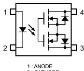
2: CATHODE 3: DRAIN 4: DRAIN
