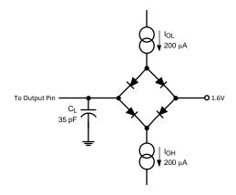
Figure 4. Timing Test Circuit
