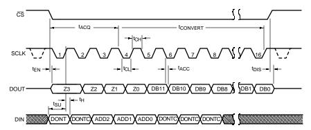
Figure 5. ADC122S101 Serial Timing Diagram
