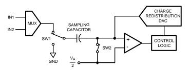
Figure 50. ADC122S101 in Hold Mode
