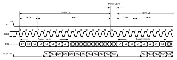
Figure 3. ADC122S101 Operational Timing Diagram
