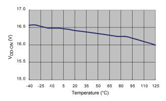
Figure 9. Start Threshold Voltage (V<sub>DD-ON</sub>) vs. Temperature
