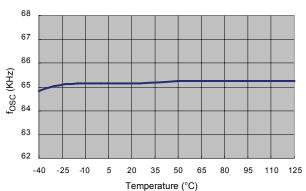
Figure 11. PWM Frequency (fosc) vs. Temperature
