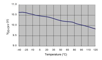
Figure 10. Minimum Operating Voltage ( $V_{\text{DD-ON}}$ ) vs. Temperature
