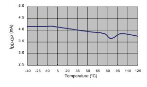
Figure 7. Operating Supply Current (I<sub>DD-OP</sub>) vs. Temperature
