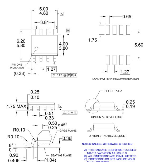
Figure 16. 8-Pin Small Outline Package (SOP)
