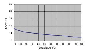
Figure 6. Startup Current (IDD-ST) vs. Temperature
