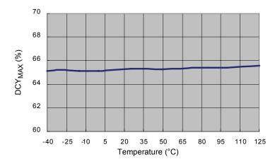
Figure 12. Maximum Duty Cycle (DCY<sub>MAX</sub>) vs. Temperature
