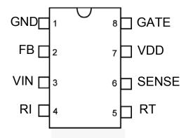
Figure 4. Pin Configuration
