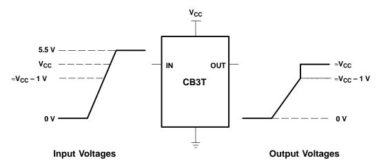
NOTE A: If the input high voltage (V<sub>IH</sub>) level is greater than or equal to V<sub>CC</sub> – 1 V, and less than or equal to 5.5 V, then the output high voltage (V<sub>OH</sub>) level will be equal to approximately the V<sub>CC</sub> voltage level.
