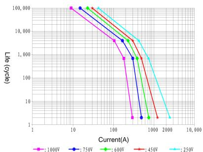
Note: Except for special note, the ambient temperature of electrical durability test is  $23^{\circ}$ C, and the on-break ratio is: 1s: 9s
