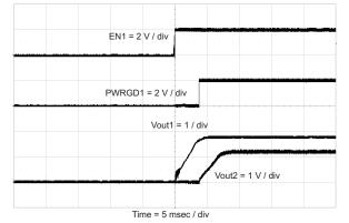
Figure 26. Sequential Startup using EN and PWRGD
