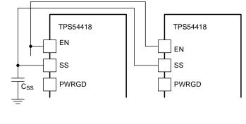
Figure 27. Ratiometric Start-Up Schematic
