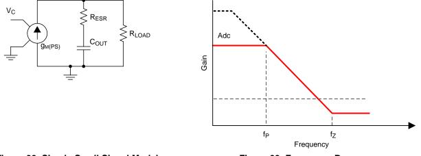
Figure 32. Simple Small Signal Model
