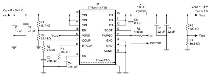
Figure 35. Typical Application Schematic, TPS54418
