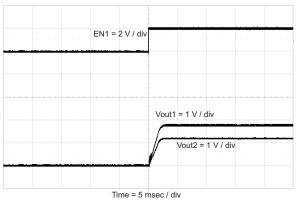
Figure 28. Ratiometric Start-Up Using Coupled SS Pins
