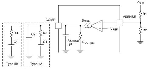
Figure 34. Types of Frequency Compensation
