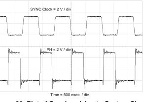
Figure 29. Synchronizing to a System Clock
