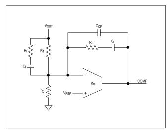
Figure 5. Type III Compensation Network
