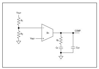
Figure 4. Type II Compensation Network
