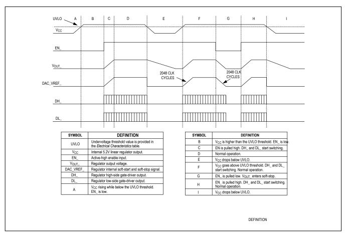
Figure 1. MAX15023 Detailed Power-On/-Off Sequencing
