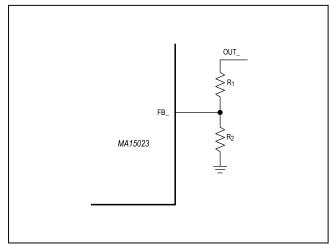
Figure 3. Adjustable Output Voltage
