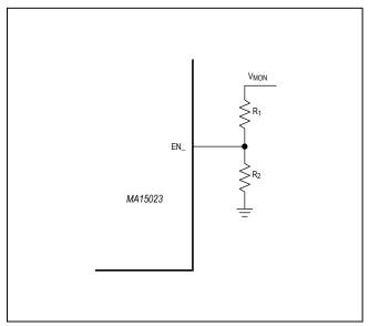
Figure 2. Adjustable Enable Voltage
