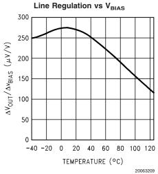
**Typical Performance Characteristics** Unless otherwise specified:  $T_A = 25^{\circ}C$ ,  $C_{OUT} = 4.7\mu F$ , Cin =  $4.7\mu F$ ,  $\overline{S/D}$  pin is tied to  $V_{BIAS}$ ,  $V_{IN} = 2.2V$ ,  $V_{OUT} = 1.8V$ . (Continued)
