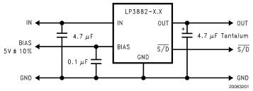
At least 4.7  $\mu\text{F}$  of input and output capacitance is required for stability.
