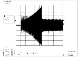
Waveform 1. Lamp filament voltage during preheat
