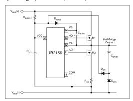
Figure 1, Start-up and supply circuitry.
