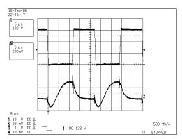
Waveform 3, Half-bridge and current sense voltage during run mode
