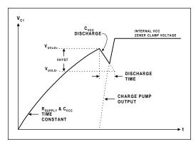
Figure 2, Supply capacitor (CVCC) voltage.
