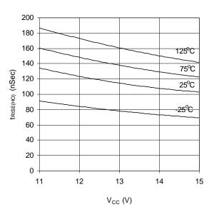
Graph 23.  $t_{RISE(HO)}$  vs  $V_{CC}$  vs Temperature (IR2156)
