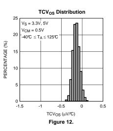
Offset Voltage vs. Temperature
