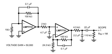
Figure 45. 0.1 Hz to 10 Hz Noise Test Circuit
