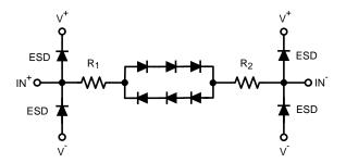
Figure 48. Anti-Parallel Diodes between Inputs
