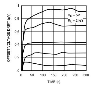
Figure 47. Start-Up Input Offset Voltage Drift
