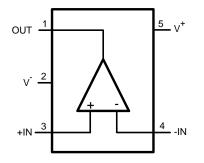
Figure 3. 5-Pin SOT-23 Top View
