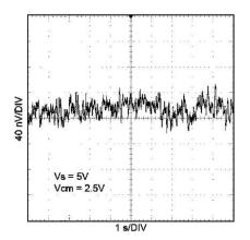
Figure 46. 0.1 Hz to 10 Hz Input Voltage Noise
