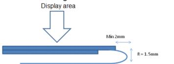
(12) The module should be fixed balanced into the housing, or the module may be twisted.
