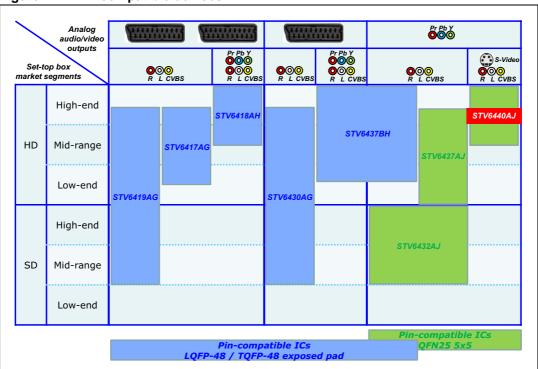
Figure 1. Pin-compatible devices
