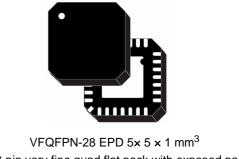
(28-pin very fine quad flat pack with exposed pad down)
