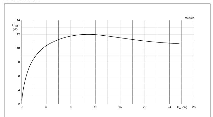
Fig.23 Total power dissipation as a function of output power;  $V_P = 14.4 \text{ V}$ ,  $R_L = 4 \Omega$  (1 channel driven BTL or 4 channels in single-ended mode).
