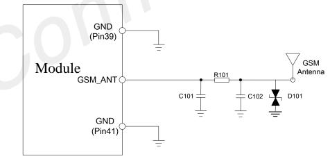
Figure 47: GSM simple antenna matching circuit
