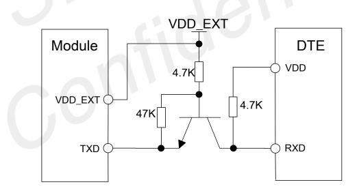
Figure 23: TX level matching circuit
