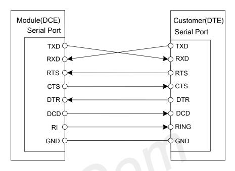
Figure 20: Connection of the serial interfaces
