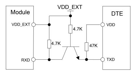
Figure 24: RX level matching circuit
