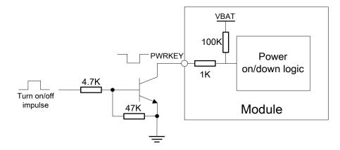
Figure 10: Powered on/off module using transistor
