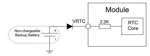
Figure 18: RTC supply from non-chargeable battery
