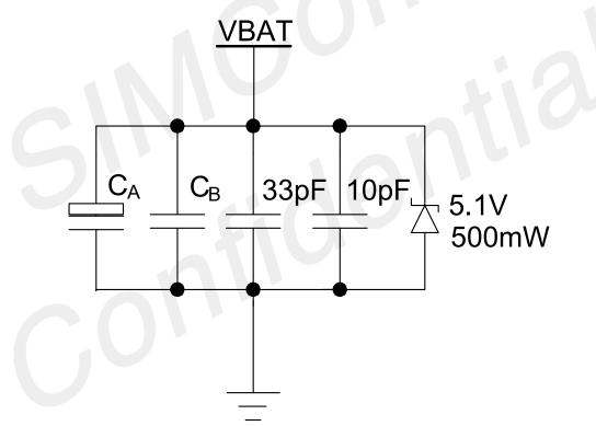
Figure 5: Reference circuit of the VBAT input
