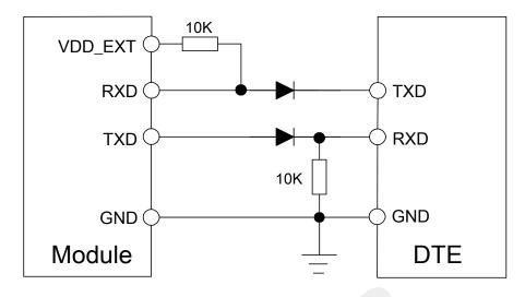
Figure 22: Diode isolation circuit
