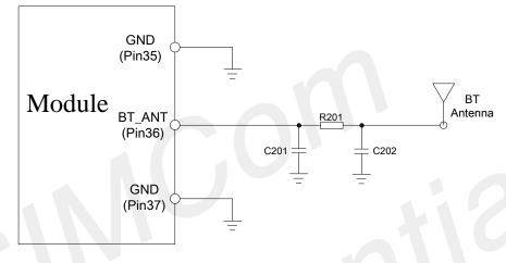
Figure 48: Bluetooth antenna matching circuit
