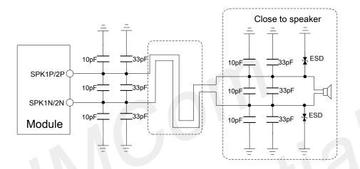
Figure 30: Speaker reference circuit
