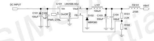
Figure 7: Reference circuit of the DC-DC power supply
