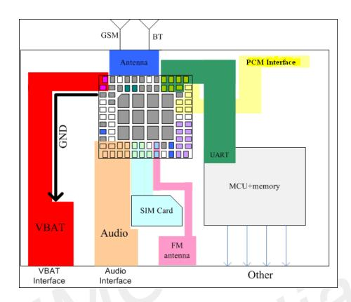
Figure 52: Recommended PCB layout
