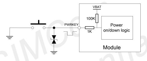
Figure 11: Powered on/off module using button
