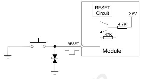
Figure 15: Reset circuit
