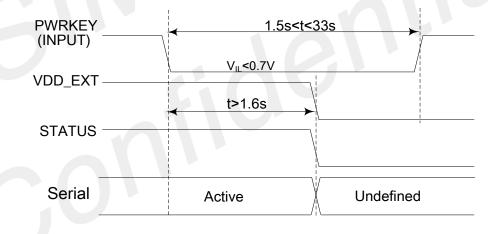
Figure 13: Timing of power down SIM800H by PWRKEY
