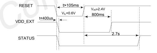
Figure 16: Reset timing sequence
