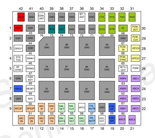
Figure 2: Pin assignment (Top view)
