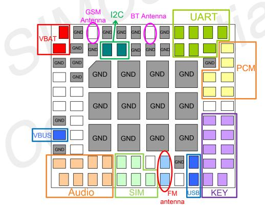
Figure 51: Pin assignment
