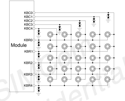
Figure 37: 25 keys reference circuit
