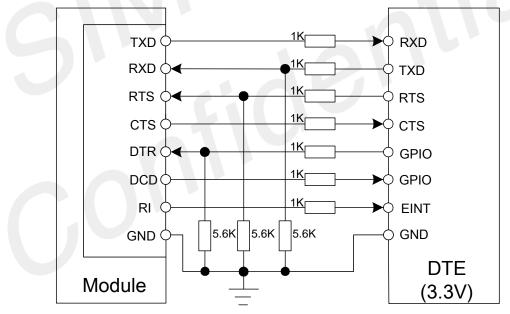
Figure 21: Resistor matching circuit
