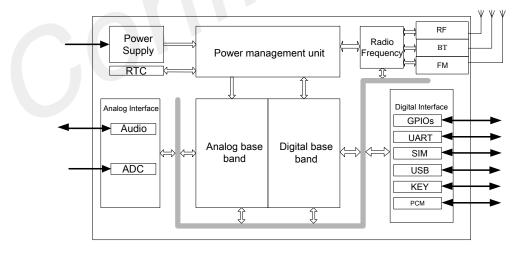
Figure 1: SIM800H functional diagram
