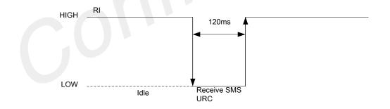
Figure 28: RI behaviour of URC or receive SMS
