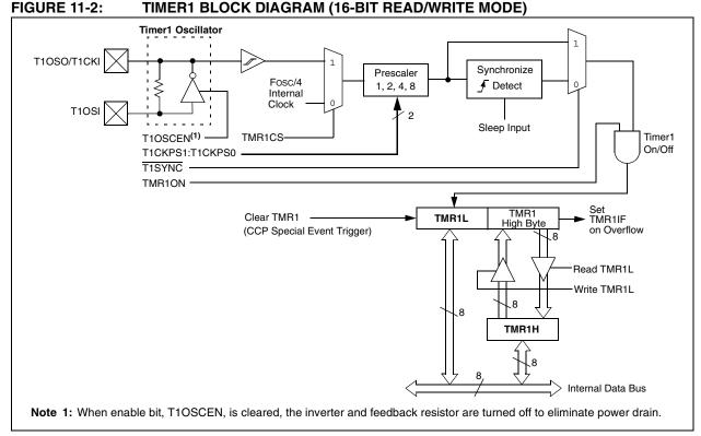
cycle (Fosc/4). When the bit is set, Timer1 increments on every rising edge of the Timer1 external clock input or the Timer1 oscillator, if enabled.
