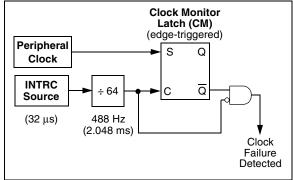
Clock failure is tested for on the falling edge of the sample clock. If a sample clock falling edge occurs while CM is still set, a clock failure has been detected (Figure 18-4). This causes the following:
