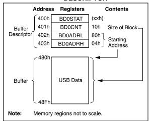
Unlike other control registers, the bit configuration for the BDnSTAT register is context sensitive. There are two distinct configurations, depending on whether the microcontroller or the USB module is modifying the BD and buffer at a particular time. Only three bit definitions are shared between the two.
