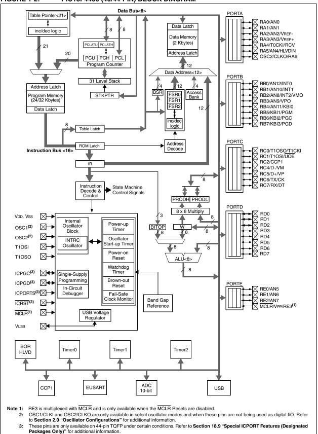
FIGURE 1-2: PIC18F4450 (40/44-PIN) BLOCK DIAGRAM
