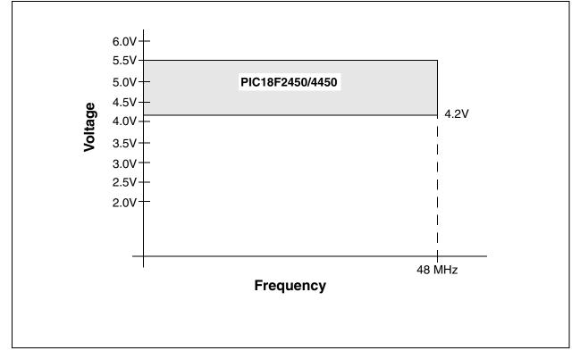
FIGURE 21-2: PIC18LF2450/4450 VOLTAGE-FREQUENCY GRAPH (INDUSTRIAL)
