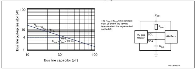
Figure 13. Maximum  $R_{bus}$  value versus bus parasitic capacitance ( $C_{bus}$ ) for an  $I^2C$  bus at maximum frequency  $f_c = 400 \text{ kHz}$
