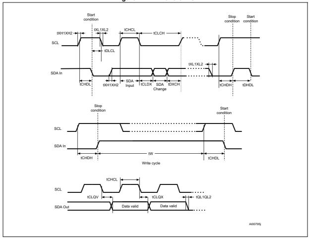
Figure 11. AC waveforms
