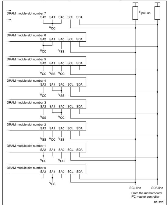
Figure 9. Serial presence detect block diagram
