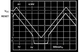
Figure 7. CBM707/CBM708 RESET Output vs.Supply Voltage
