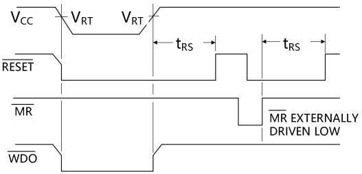
Figure 13. RESET, MR, and WDO Timing
