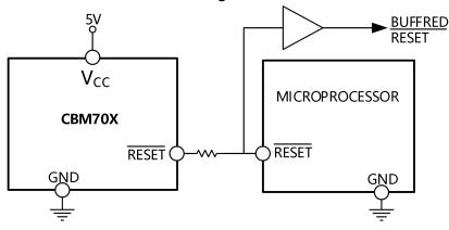
Figure 21. Bidirectional Input/Output RESET
