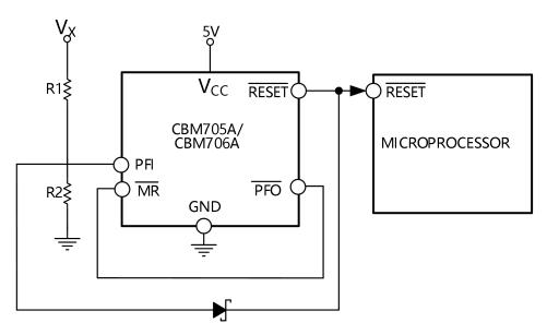
Figure 20. Monitoring 5 V and an Additional Supply, VX
