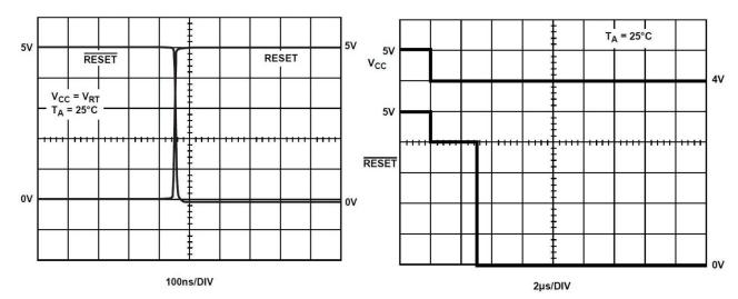
Figure 10. RESET ,RESET Assertion
