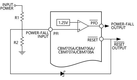
Figure 15. Power Fail Comparator
