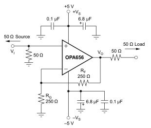
Figure 29. Noninverting G = +2 V/V Specifications and Test Circuit
