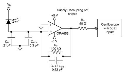
Figure 32. Wideband, High-Sensitivity, Transimpedance Amplifier
