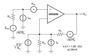
Figure 31. Operational Amplifier Noise Analysis Model
