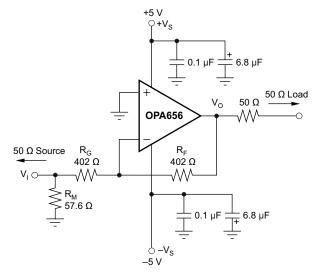
Figure 30. Inverting G = -1 V/V Specifications and Test Circuit
