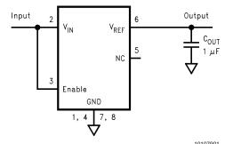
$C_{\mbox{\scriptsize OUT}},$  Output bypass capacitor. See text for selection detail.
