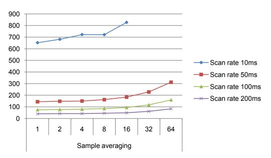
Figure 32-11. Power Consumption [µA] 100 sensors, noise countermeasures disabled, f=48MHz, Vcc=3.3V
