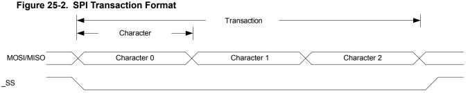
The SPI master must pull the slave select line ( $\overline{SS}$ ) of the desired slave low to initiate a transaction. The master and slave prepare data to send via their respective shift registers, and the master generates the serial clock on the SCK line.
