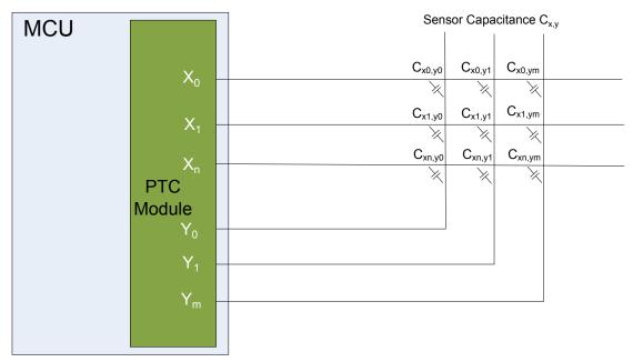
Figure 31-3. Mutual Capacitance Sensor Arrangement
