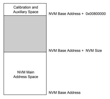
The lower rows in the NVM main address space can be allocated as a boot loader section by using the BOOTPROT fuses, and the upper rows can be allocated to EEPROM, as shown in the figure below.
