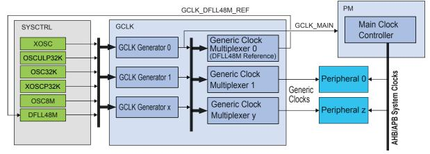
The clock system on the SAM D20 consists of:
