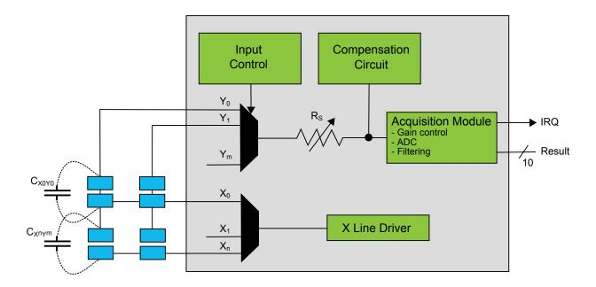
Figure 31-2. PTC Block Diagram Self-Capacitance
