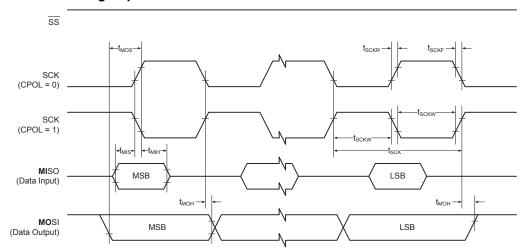
Figure 32-15. SPI timing requirements in slave mode
