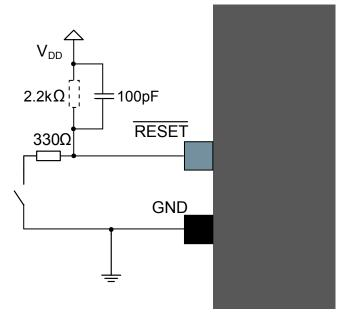
A pull-up resistor makes sure that the reset does not go low and unintentionally cause a device reset. An additional resistor has been added in series with the switch to safely discharge the filtering capacitor, i.e., preventing a current surge when shorting the filtering capacitor which again can cause a noise spike that can have a negative effect on the system.
