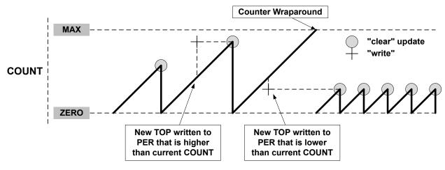
Figure 27-7. Changing the Top value with Up-Counting Operation
