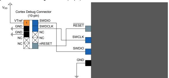
Table 35-10. Cortex Debug Connector (10-pin)
