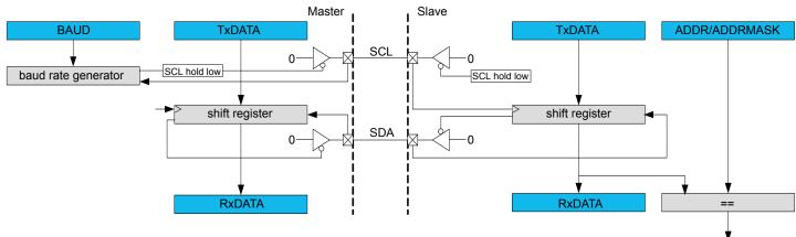
Figure 26-1. I<sup>2</sup>C Single-Master Single-Slave Interconnection
