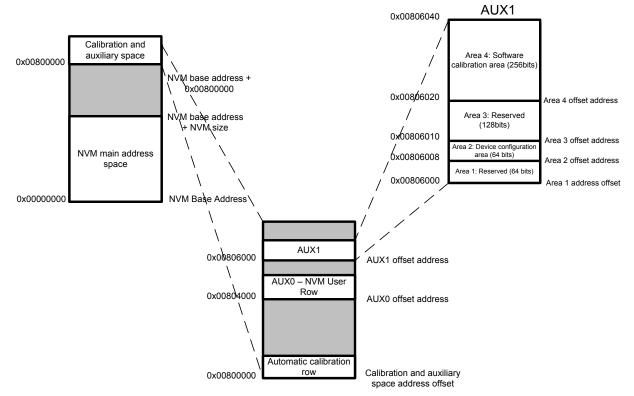
Figure 9-1. Calibration and Auxiliary Space
