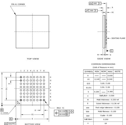
Notes : 1. This drawing is for general information only. Refer to JEDEC Drawing MO-280, Variation UCCBB for proper dimensions, tolerances, datums, etc. 2. Array as seen from the bottom of the package.
