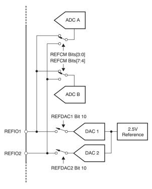
Figure 29. Reference Selection Circuit
