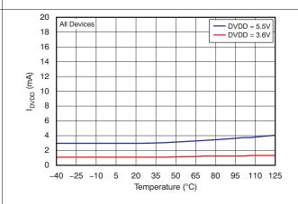
Figure 23. Analog Supply Current vs Temperature
