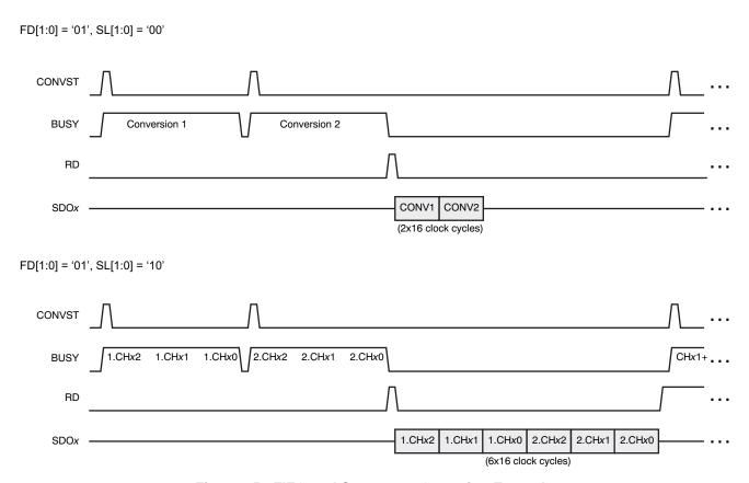
Figure 45. FIFO and Sequencer Operation Example
