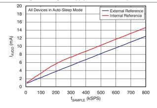
Figure 25. Analog Supply Current vs Data Rate
