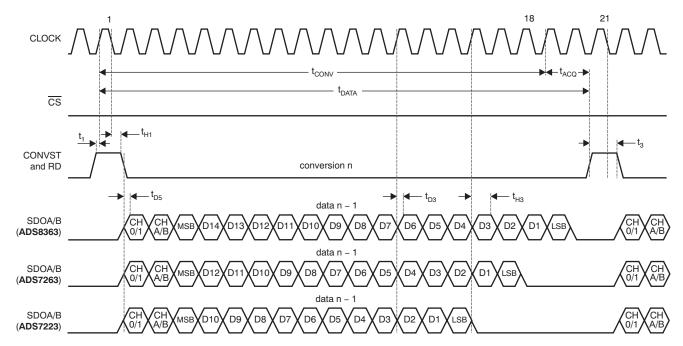
Figure 48. Four-Wire Application Timing (Half-Clock Mode)
