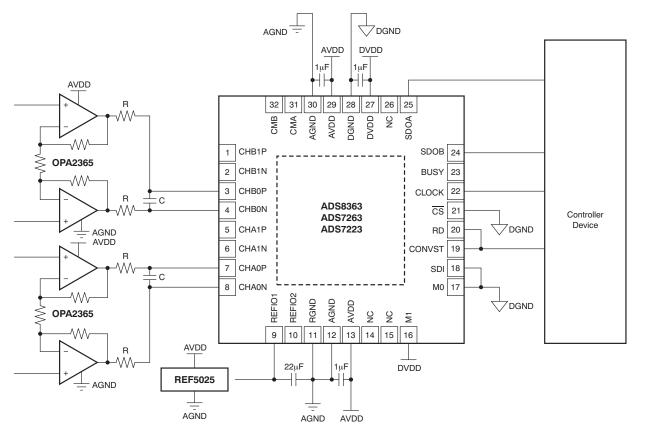
Figure 47. Four-Wire Application Configuration
