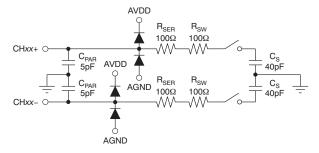
Figure 28. Equivalent Analog Input Circuit
