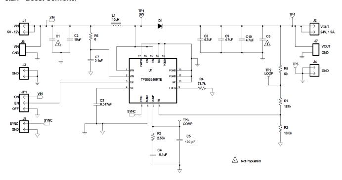
Figure 16. Boost Converter Application Schematic
