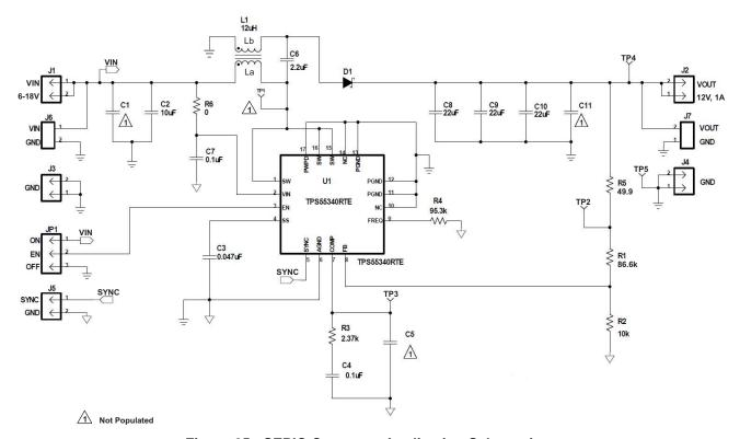
Figure 25. SEPIC Converter Application Schematic
