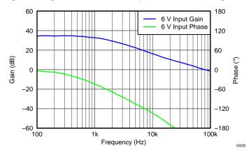
Figure 26. SEPIC Power Stage Gain and Phase
