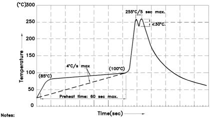
1.Recommend pre—heat temperature of 105°C or less (as measured with a thermocouple attached to the LED pins) prior to immersion in the solder wave with a maximum solder bath temperature of 260°C
