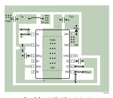
Figure 5. Suggested Boost Converter Layout
