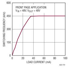
Figure 1. Burst Frequency vs Load Current
