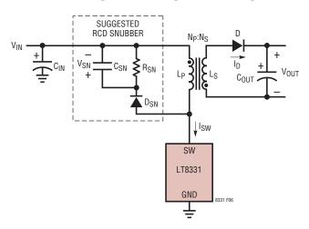
Figure 6. A Simplified Flyback Converter
