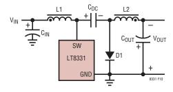
Figure 10. A Simplified Inverting Converter
