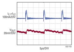
Figure 2. Burst Mode Operation
