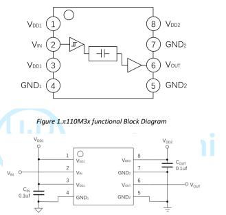
Figure 2.π110M3x Typical Application Circuit
