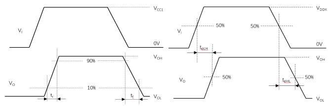
Figure 7.Transition time waveform measurement
