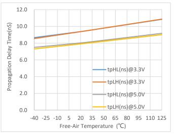
Figure 6. Propagation Delay Time vs. Free-Air Temperature
