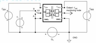
Figure 11.Common-mode transient immunity (CMTI) measurement
