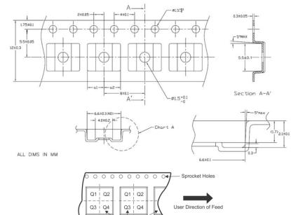
Note: The Pin 1of the chip is in the quadrant Q1 Figure 15.NB SOIC-8 Reel Information-dimension unit(mm)
