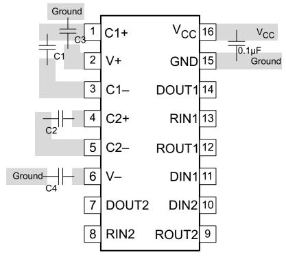
Figure 8. Layout Diagram
