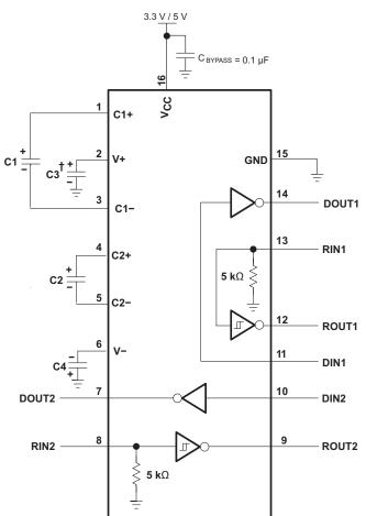
$\dagger$  C3 can be connected to  $V_{CC}$  or GND.
