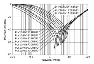
Differential Mode Insertion Loss (Typ.)
