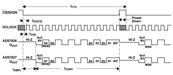
Figure 37. ADS7826 and ADS7827 Timing
