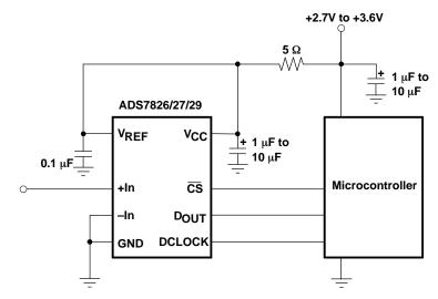
Figure 40. Basic Data Acquisition System
