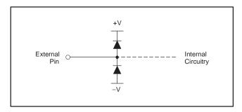
Figure 2. ESD Protection Diodes
