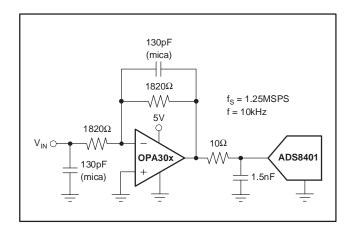
Figure 4. The OPA30x Drives the 16-Bit ADS8401
