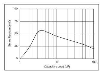
Figure 3. Recommended R<sub>S</sub> and C<sub>L</sub> Combinations
