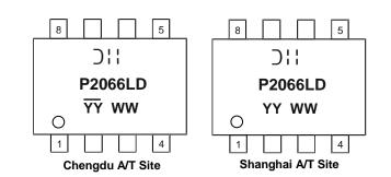
);; = Manufacturer's Marking P2066LD = Product Type Marking Code YYWW = Date Code Marking YY or  $\overrightarrow{YY}$  = Year (ex: 18 = 2018) WW = Week (01 to 53)  $\overrightarrow{YY}$  = Date Code Marking for SAT (Shanghai Assembly/ Test Site)  $\overrightarrow{YY}$  = Date Code Marking for CAT (Chengdu Assembly/ Test Site)
