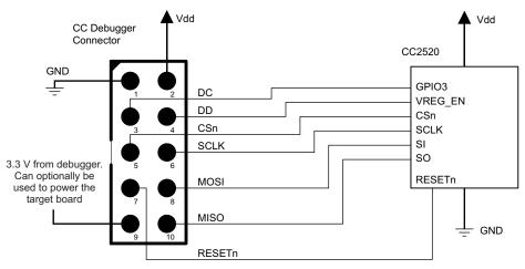
Figure 8. CC Debugger Connected to CC2520
