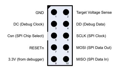
Figure 4. Target Connector Pin-Out
