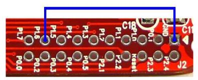
Figure 17. Short-Circuit Pins for Boot Recovery Mode
