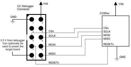
Figure 11. CC Debugger Connected to CC85XX
