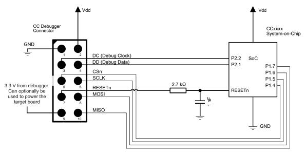
Figure 7. Connection to SoC to Enable Packet Sniffing
