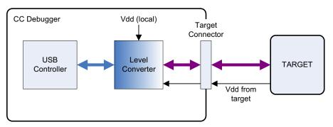
Figure 5. Voltage From Target to CC Debugger
