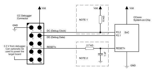
Figure 6. Minimum Connection for Debugging of 8051 SoC
