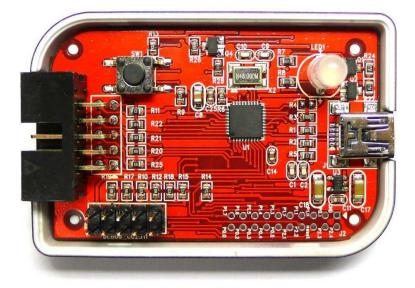
Figure 16. Internal View of CC Debugger
