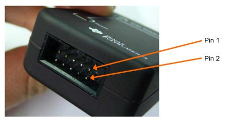
Figure 2. Placement of Target Connector Pins
