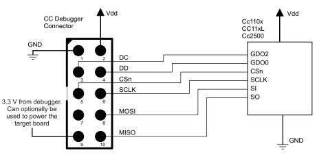
Figure 10. CC Debugger Connected to CC110x/CC11xL/CC2500
