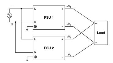
Fig. 10 Parallel Operation Connection Diagram
