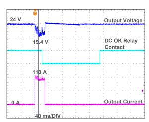
Fig. 8.2 APB 275% of nominal output current for 25 ms
