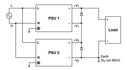
Fig. 11 Series Operation Connection Diagram
