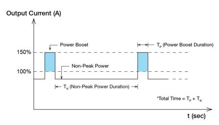
Fig. 7 Duty Cycle Calculation
