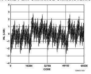
Figure 5. Integral Nonlinearity vs. Code
