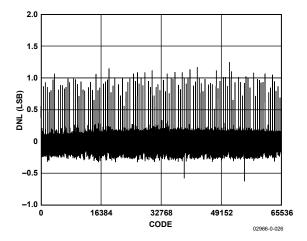
Figure 8. Differential Nonlinearity vs. Code
