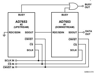
Figure 36. Two AD7653s in a Daisy-Chain Configuration
