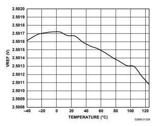
Figure 17. Typical Reference Output Voltage vs. Temperature
