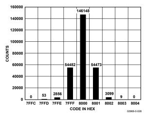
Figure 9. Histogram of 261,120 Conversions of a DC Input at the Code Center
