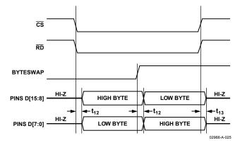
Figure 31. 8-Bit Parallel Interface
