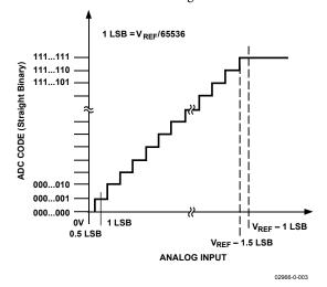
Figure 21. ADC Ideal Transfer Function
