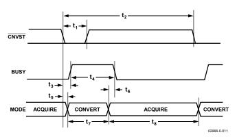
Figure 26. Basic Conversion Timing
