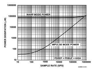
Figure 25. Power Dissipation vs. Sampling Rate
