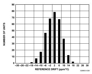
Figure 18. Reference Voltage Temperature Coefficient Distribution (335 Units)
