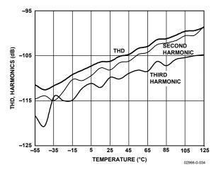
Figure 14. THD and Harmonics vs. Temperature
