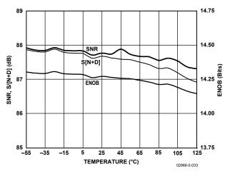
Figure 13. SNR, S/(N+D), and ENOB vs. Temperature
