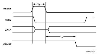
Figure 27. RESET Timing
