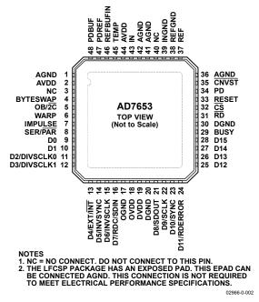
Figure 4. 48-Lead LQFP (ST-48) and 48-Lead LFCSP (CP-48-1)
