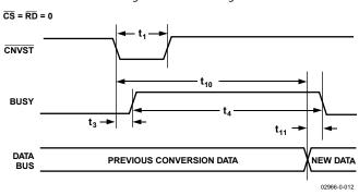
Figure 28. Master Parallel Data Timing for Reading (Continuous Read)
