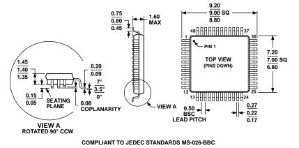
Figure 39. 48-Lead Quad Flat Package [LQFP] (ST-48) Dimensions shown in millimeters
