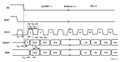
Figure 34. Slave Serial Data Timing for Reading (Read after Convert)
