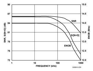
Figure 10. SNR, S/(N+D), and ENOB vs. Frequency
