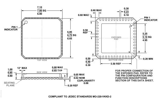
Figure 40. 48-Lead Lead Frame Chip Scale Package [LFCSP] 7 mm × 7 mm Body and 0.85 mm Package Height
