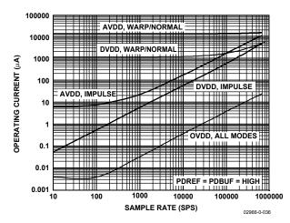
Figure 15. Operating Current vs. Sample Rate
