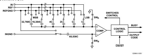
Figure 20. ADC Simplified Schematic
