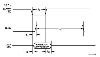
Figure 30. Slave Parallel Data Timing for Reading (Read during Convert Mode)
