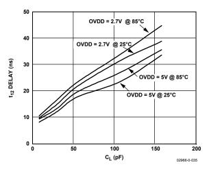
Figure 19. Typical Delay vs. Load Capacitance CL
