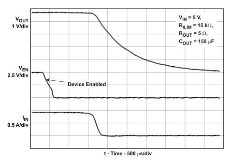
Figure 6. Turnoff Delay and Fall Time
