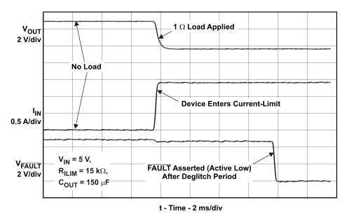
Figure 12. No Load to 1Ω Transient Response
