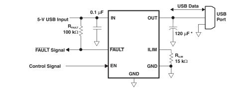
$^{\ast}$  USB requirement that downstream-facing ports are bypassed with at least 120  $\mu F$  per hub
