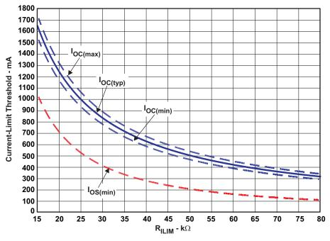
Figure 21. Current-Limit Threshold vs RILIM
