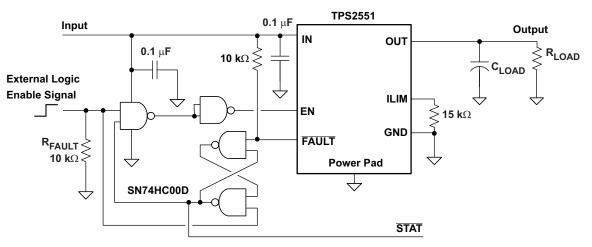
Figure 24. Overcurrent Latch-Off Using a Quad-NAND Gate
