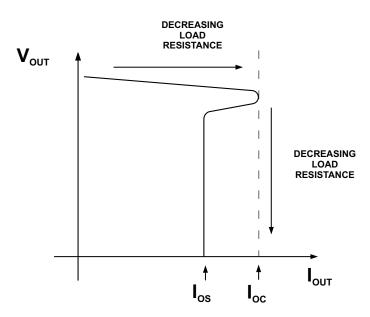
Figure 4. Output Voltage vs. Current-Limit Threshold
