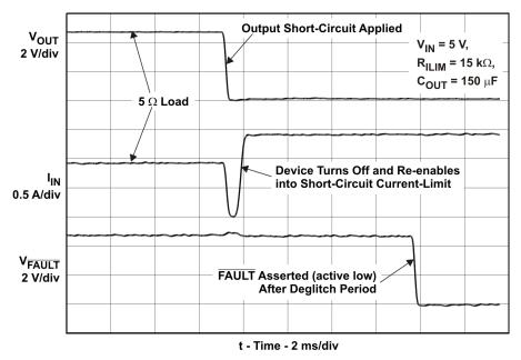
Figure 8. Full-Load to Short-Circuit Transient Response
