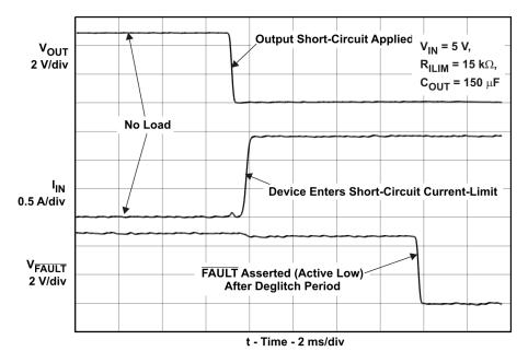
Figure 10. No-Load to Short-Circuit Transient Response
