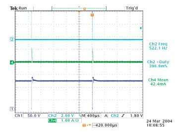
0.4% PWM Ratio at 500Hz Dimming
