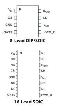
No Connects (NC) are not internally connected and may be used for pass-thru PCB traces.
