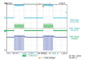
33% PWM Ratio at 500Hz Dimming
