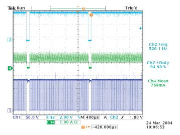
95% PWM Ratio at 500Hz Dimming
