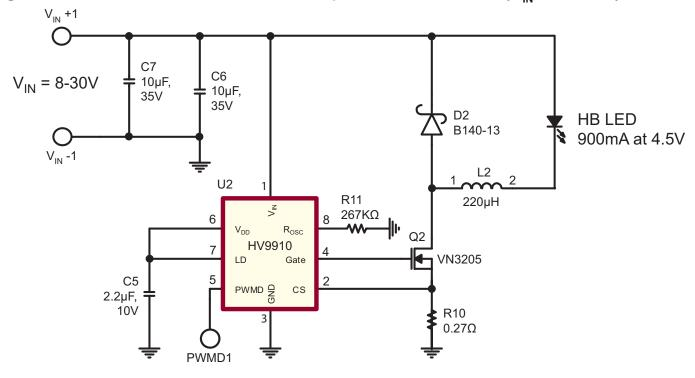
Figure 3: HV9910 Buck-Boost driver powering 3 to 8, 350mA HB LEDs ( $V_{IN}$  = 8 - 30V)
