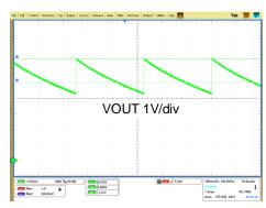
Figure 5. Low voltage and light load, BST-UVLO operation waveform VOUT=5V VCC=7V IOUT=0mA
