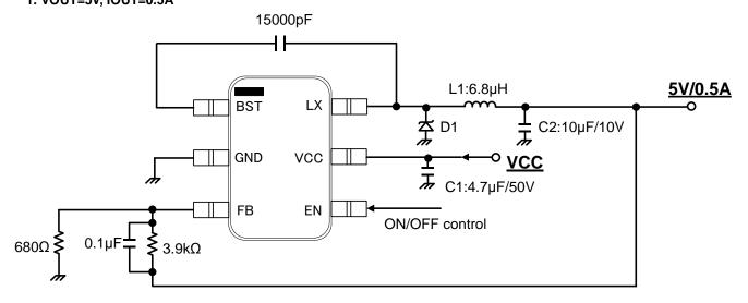
Figure 19. Typical Application Circuit (VOUT=5V)
