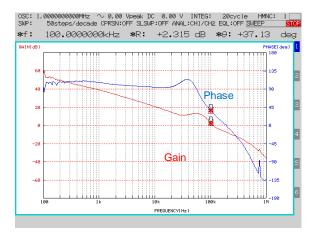
Figure 44. Frequency Response IOUT=500mA, VOUT=12V
