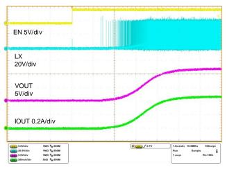
Figure 39. Start-up Characteristics VCC=42V, IOUT=500mA, VOUT=12V
