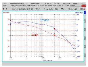
Figure 30. Frequency Response IOUT=100mA, VOUT=5V
