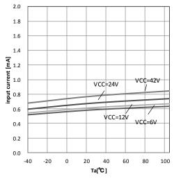
Figure 9. Operating Current - Temperature
