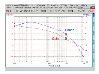
Figure 43. Frequency Response IOUT=100mA, VOUT=12V
