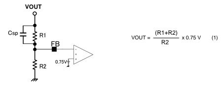
Figure 6. Voltage feedback resistance setting
