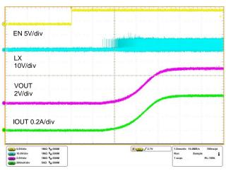
Figure 22. Start-up Characteristics VCC=8V, IOUT=500mA, VOUT=5V
