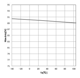
Figure 12. Max Duty - Temperature
