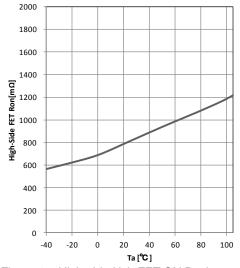
Figure 15. High-side Nch-FET ON Resistance - Temperature
