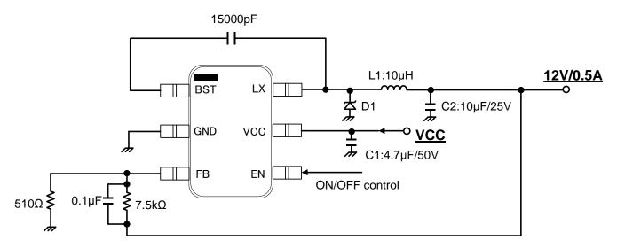
Figure 32. Typical Application Circuit (VOUT=12V)
