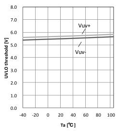
Figure 10. UVLO Threshold - Temperature
