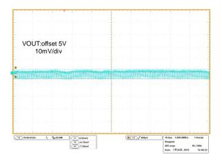
Figure 29. VOUT Ripple IOUT=200mA, VOUT=5V
