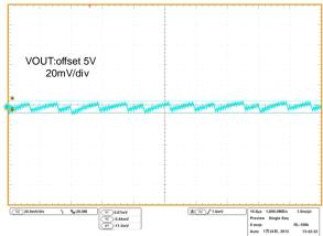
Figure 41. VOUT Ripple IOUT=50mA, VOUT=12V
