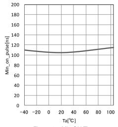
Figure 17. Min ON Time - Temperature
