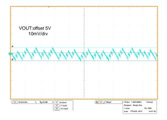
Figure 28. VOUT Ripple IOUT=20mA, VOUT=5V
