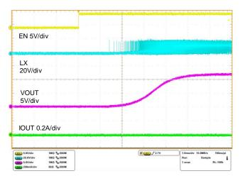
Figure 34. Start-up Characteristics VCC=18V, IOUT=0mA, VOUT=12V
