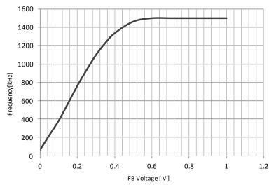
Figure 7. FB voltage -frequency Characteristics
