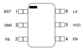
Figure 2. Pin Configuration (TOP VIEW)
