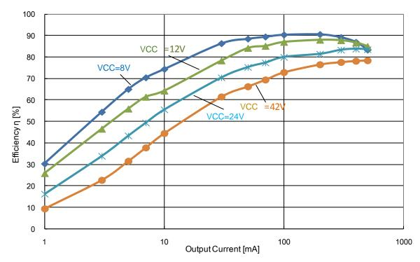
Figure 20. Power Conversion Efficiency - Output Current VOUT=5V
