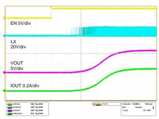
Figure 35. Start-up Characteristics VCC=18V, IOUT=500mA, VOUT=12V
