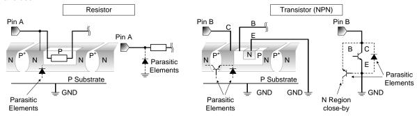
Figure 50. Example of monolithic IC structure
