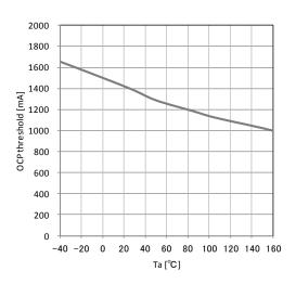
Figure 16. OCP threshold-Temperature
