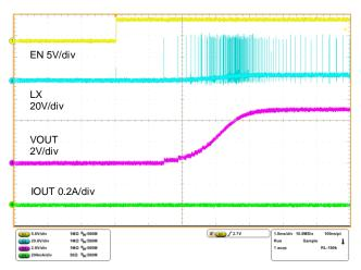
Figure 25. Start-up Characteristics VCC=42V, IOUT=0mA, VOUT=5V
