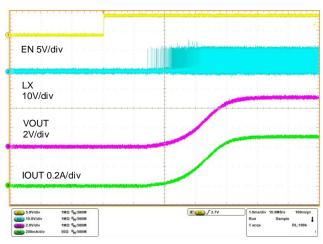
Figure 24. Start-up Characteristics VCC=12V, IOUT=500mA, VOUT=5V
