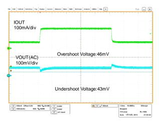
Figure 27. Load Response IOUT=50mA<->200mA, VOUT=5V
