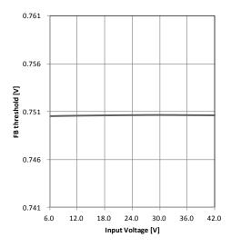
Figure 13. FB Pin Reference Voltage - Input Voltage
