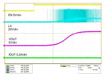
Figure 38. Start-up Characteristics VCC=42V, IOUT=0mA, VOUT=12V
