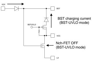
Figure 4. BST-UVLO equivalent circuit
