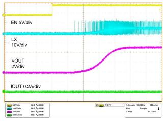
Figure 23. Start-up Characteristics VCC=12V, IOUT=0mA, VOUT=5V
