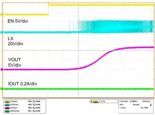
Figure 36. Start-up Characteristics VCC=24V, IOUT=0mA, VOUT=12V
