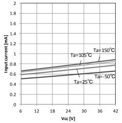
Figure 8. Operating Current - Input Voltage
