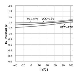
Figure 18. EN Threshold Voltage - Temperature
