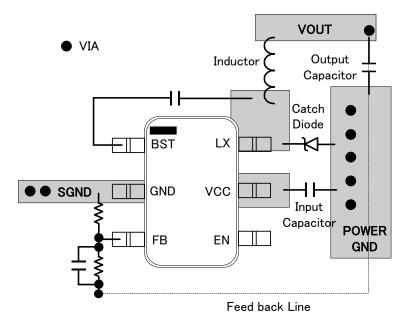
Figure 47. Reference PCB layout
