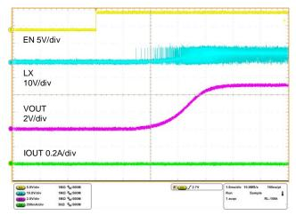
Figure 21. Start-up Characteristics VCC=8V, IOUT=0mA, VOUT=5V
