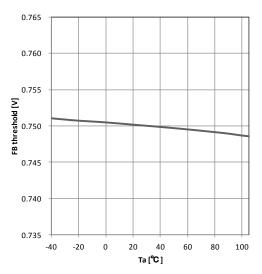
Figure 14. FB Threshold - Temperature
