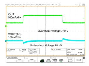
Figure 40. Load Response IOUT=50mA<->200mA, VOUT=12V
