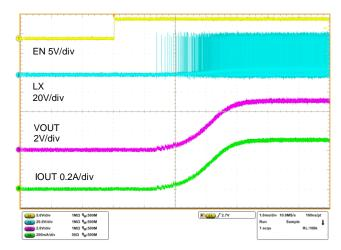
Figure 26. Start-up Characteristics VCC=42V, IOUT=500mA, VOUT=5V
