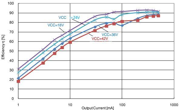
\*The efficiency falls when the switching waveform is turning from intermittent mode to continuous mode
