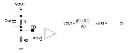
Figure 46. Voltage feedback resistance setting
