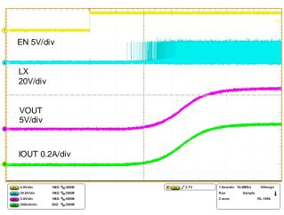
Figure 37. Start-up Characteristics VCC=24V, IOUT=500mA, VOUT=12V
