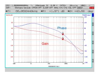
Figure 31. Frequency Response IOUT=500mA, VOUT=5V
