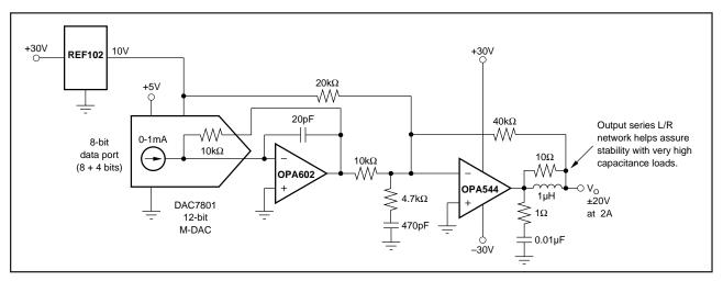
FIGURE 5. Digitally Programmable Power Supply.
