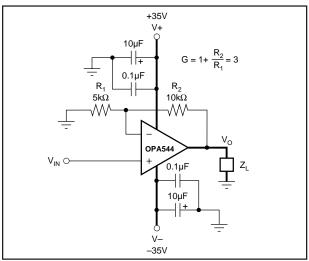
FIGURE 1. Basic Circuit Connections.
