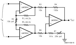
FIGURE 10. Instrumentation Amplifier
