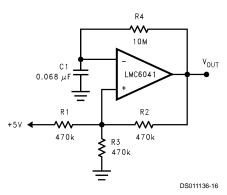
FIGURE 11. 1 Hz Square-Wave Oscillator
