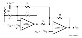
FIGURE 7. Two Op-Amp Instrumentation Amplifier
