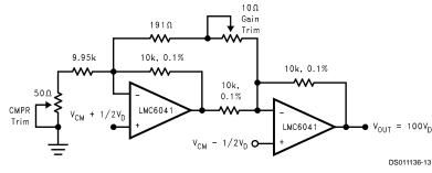
FIGURE 8. Low-Power Two-Op-Amp Instrumentation Amplifier
