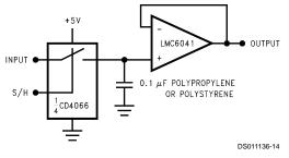
FIGURE 9. Low-Leakage Sample and Hold
