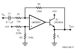
FIGURE 12. AC Coupled Power Amplifier
