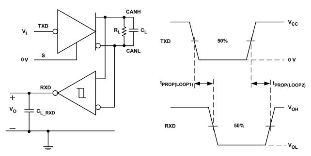
Figure 9. T<sub>PROP(LOOP)</sub> Test Circuit and Measurement
