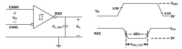
Figure 4. RXD Dominant Timeout Test Circuit and Measurement
