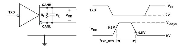
Figure 10. TXD Dominant Timeout Test Circuit and Measurement
