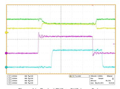
Figure 21. Typical TXD to RXD Loop Delay
