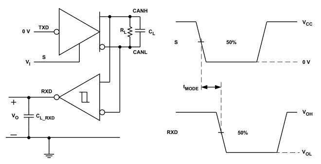
Figure 8.  $t_{\text{MODE}}$  Test Circuit and Measurement
