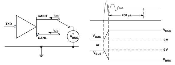
Figure 11. Driver Short Circuit Current Test and Measurement
