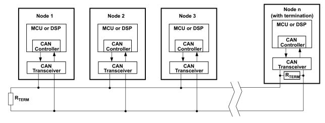
Figure 18. Typical CAN Bus
