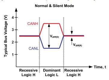
Figure 15. Bus States (Physical Bit Representation)
