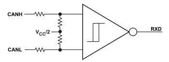
Figure 16. Simplified Recessive Common Mode Bias and Receiver
