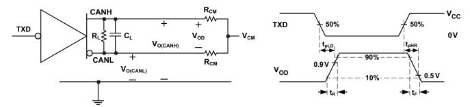
Figure 6. Driver Test Circuit and Measurement
