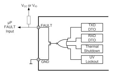
Figure 12. FAULT Pin Function Diagram and Application
