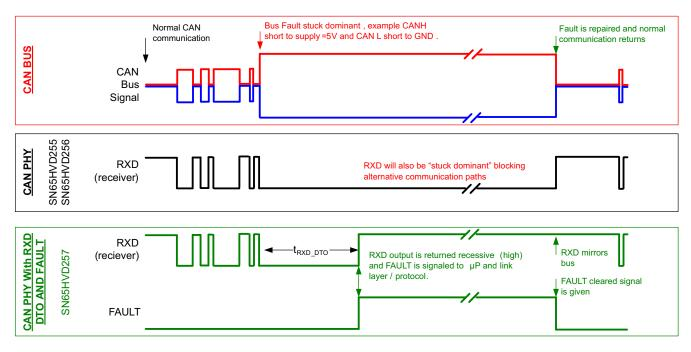
Figure 14. Example Timing Diagram for Devices With and Without RXD DTO and FAULT Pin
