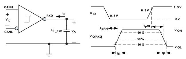
Figure 7. Receiver Test Circuit and Measurement
