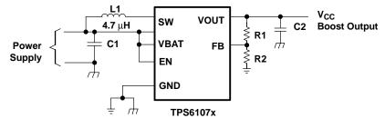
List of Components: U1 = TPS61070DDC L1 = Wurth Elektronik 744031004 C1 = 2 x 4.7  $\mu$ F, 0603, X7R/X5R Ceramic C2 = 2 x 4.7  $\mu$ F, 0603, X7R/X5R Ceramic
