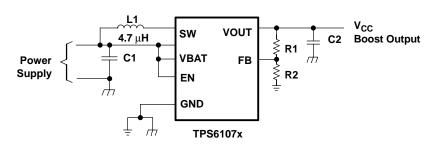
List of Components: U1 = TPS61070DDC L1 = Taiyo Yuden CB2016B4R7M C1 = 1 x 4.7 μF, 0603, X7R/X5R Ceramic C2 = 2 x 4.7 μF, 0603, X7R/X5R Ceramic
