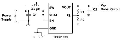
List of Components: U1 = TPS61070DDC L1 = Wurth Elektronik 744031004 C1 = 2 x 4.7 µF, 0603, X7R/X5R Ceramic C2 = 4 x 4.7 µF, 0603, X7R/X5R Ceramic
