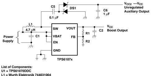
U1 = TPS61070DDC L1 = Wurth Elektronik 744031004 C1 = 2 x 4.7 μF, 0603, X7R/X5R Ceramic C2 = 2 x 4.7 μF, 0603, X7R/X5R Ceramic
