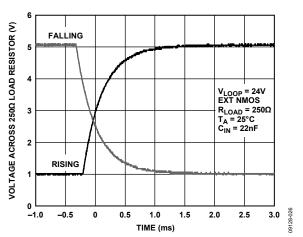
Figure 27. Full-Scale Loop Current Step, C<sub>IN</sub> = 22 nF
