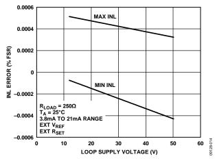
Figure 16. Integral Nonlinearity Error vs. Loop Supply Voltage
