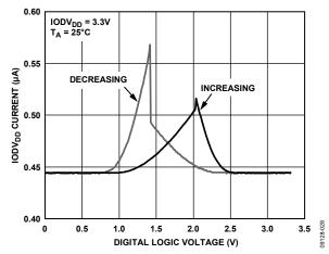
Figure 29. IODV<sub>DD</sub> Current vs. Digital Logic Voltage, Increasing and Decreasing, IODV<sub>DD</sub> = 3.3 V
