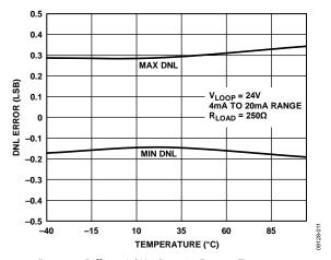
Figure 13. Differential Nonlinearity Error vs. Temperature
