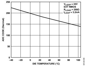
Figure 39. On-Chip ADC Code vs. Die Temperature
