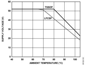
Figure 53. Maximum Supply Voltage vs. Ambient Temperature
