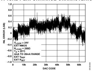
Figure 7. Integral Nonlinearity Error vs. Code
