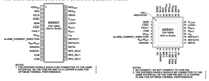
Figure 5. TSSOP Pin Configuration
