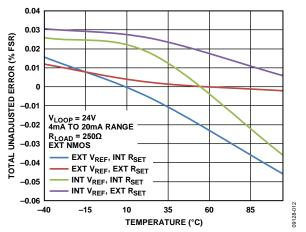
Figure 14. Total Unadjusted Error vs. Temperature
