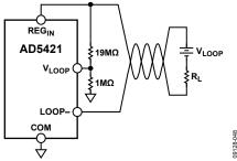
Figure 42. Resistor Divider Connection at VLOOP Pin
