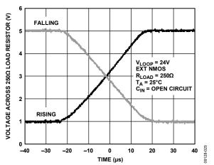
Figure 26. Full-Scale Loop Current Step
