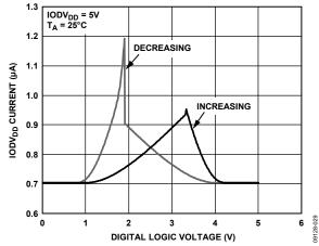
Figure 30. IODV<sub>DD</sub> Current vs. Digital Logic Voltage, Increasing and Decreasing, IODV<sub>DD</sub> = 5 V
