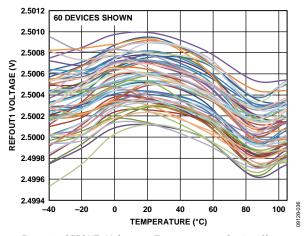
Figure 37. REFOUT1 Voltage vs. Temperature, 60 Devices Shown (C Grade Device)
