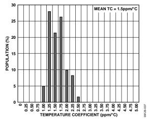
Figure 38. REFOUT1 Temperature Coefficient Histogram (C Grade Device)
