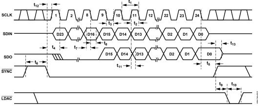
Figure 2. Serial Interface Timing Diagram
