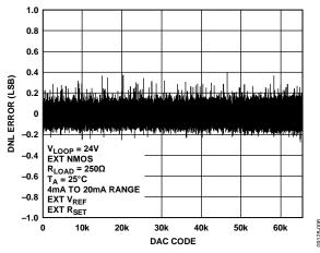
Figure 8. Differential Nonlinearity Error vs. Code
