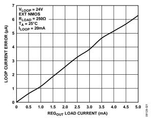
Figure 23. Loop Current Error vs. REG<sub>OUT</sub> Load Current
