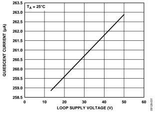
Figure 32. Quiescent Current vs. Loop Supply Voltage
