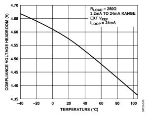
Figure 22. Compliance Voltage Headroom vs. Temperature
