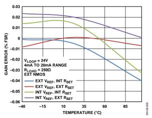
Figure 11. Gain Error vs. Temperature
