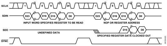
Figure 3. Readback Timing Diagram
