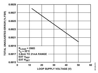
Figure 17. Total Unadjusted Error vs. Loop Supply Voltage
