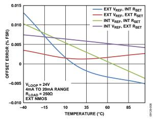
Figure 10. Offset Error vs. Temperature
