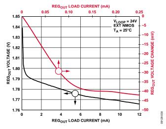
Figure 31. REGOUT Voltage vs. Load Current
