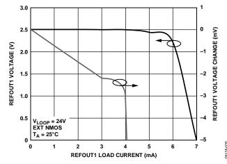
Figure 36. REFOUT1 Voltage vs. Load Current
