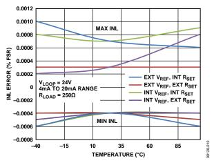
Figure 12. Integral Nonlinearity Error vs. Temperature
