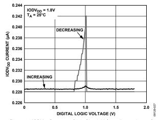
Figure 28. IODV<sub>DD</sub> Current vs. Digital Logic Voltage, Increasing and Decreasing, IODV<sub>DD</sub> = 1.8 V
