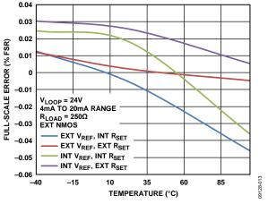
Figure 15. Full-Scale Error vs. Temperature
