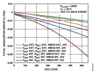
Figure 9. Total Unadjusted Error vs. Code
