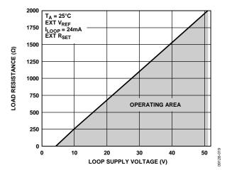
Figure 21. Load Resistance Load Line vs. Loop Supply Voltage (Voltage Between LOOP— and REG<sub>IN</sub>)
