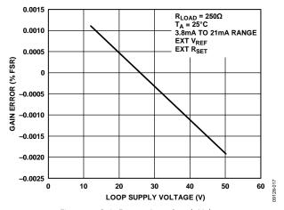
Figure 19. Gain Error vs. Loop Supply Voltage
