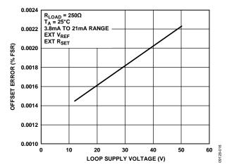
Figure 18. Offset Error vs. Loop Supply Voltage
