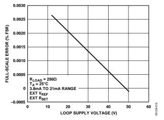
Figure 20. Full-Scale Error vs. Loop Supply Voltage
